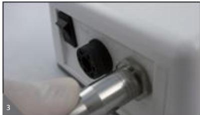
Finishing the connection of turbine hose connector.
